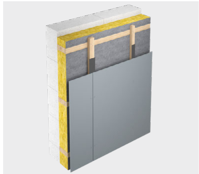
Construction with horizontal counter battens
