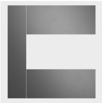
Correct mounting of Hardie® Panel & Hardie® Architectural Panel at windows, doors and openings.
