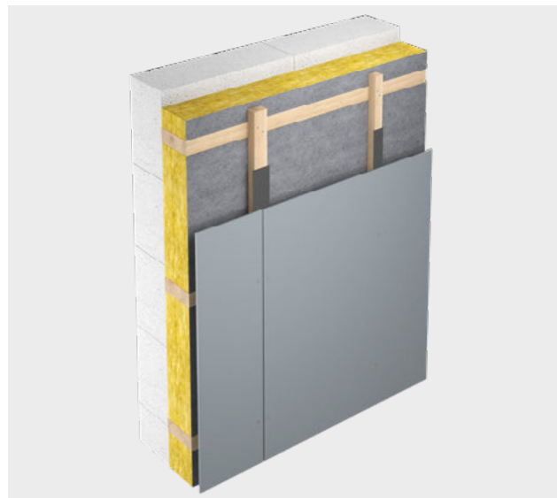
Construction with horizontal counter battens
